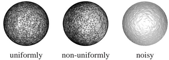
Figure 1: Meshes for spherical surface with 8000 sample points for meshes.
